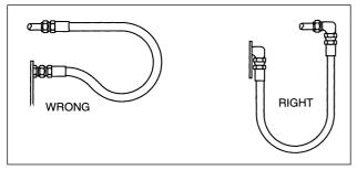
When radius is below the required minimum, use an angle adaptor to avoid sharp bends.
