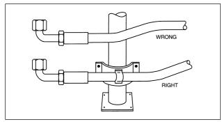
High ambient temperatures shorten hose life so make sure hose is kept away from hot parts. If this is not possible, insulate hose.
