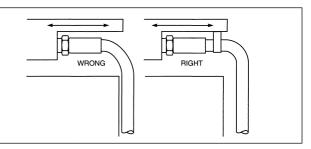
Run hose in the installation so that it avoids rubbing and abrasion. Often, clamps are required to support long hose runs or to keep hose away from moving parts. Use clamps of the correct size. A clamp too large allows hose to move inside the clamp and causes abrasion.
