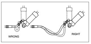
Adequate hose length is necessary to distribute movement on flexing applications and to avoid abrasion.
