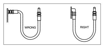
Use proper angle adaptors to avoid sharp twist or bend in hose.
