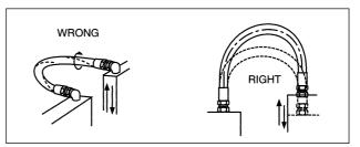
Prevent twisting and distortion by bending hose in same plane as the motion of the boss to which hose is connected.
