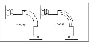
When installing hose, make sure it is not twisted. Pressure applied to a twisted hose can result in hose failure or loosening of connections.
