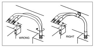
Avoid twisting of hose lines bent in two planes by clamping hose at change of plane.
