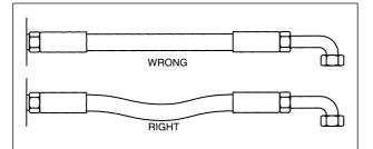
When hose installation is straight, allow enough slack in hose line to provide for length changes which will occur when pressure is applied.
