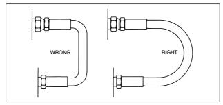
To avoid hose collapse and flow restriction, keep hose bend radii as large as possible. Refer to hose specification tables for minimum bend radii.
