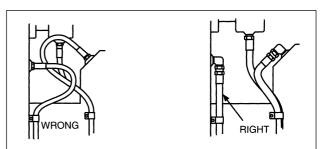
Route hose directly by using  $45^\circ$  and/or  $90^\circ$  adaptors and fittings. Avoid excessive hose length to improve appearance.
