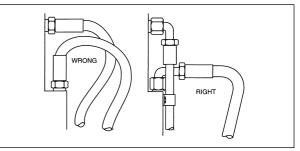
Elbows and adaptors should be used to relieve strain on the assembly, and to provide neater installations which will be more accessible for inspection and maintenance.
